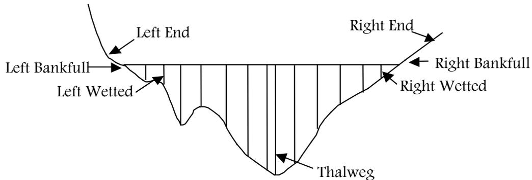
Figure 1. Example cross sectional profile with point labeling (looking downstream).
