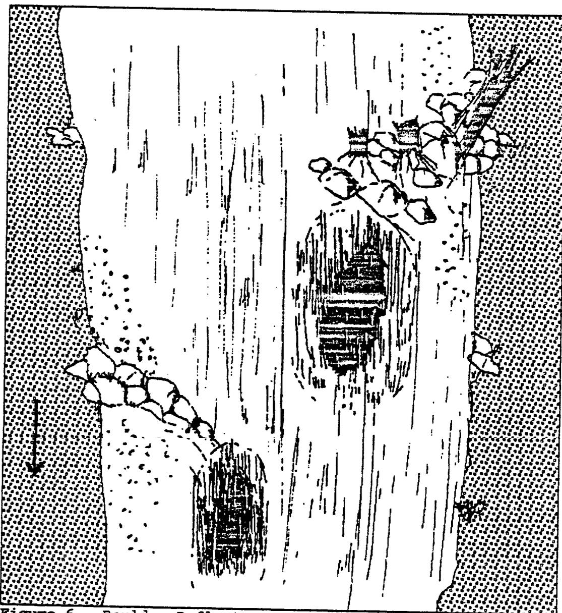
**Figure 6. Boulder Deflector and Boulder/Rootwad Deflector.**
