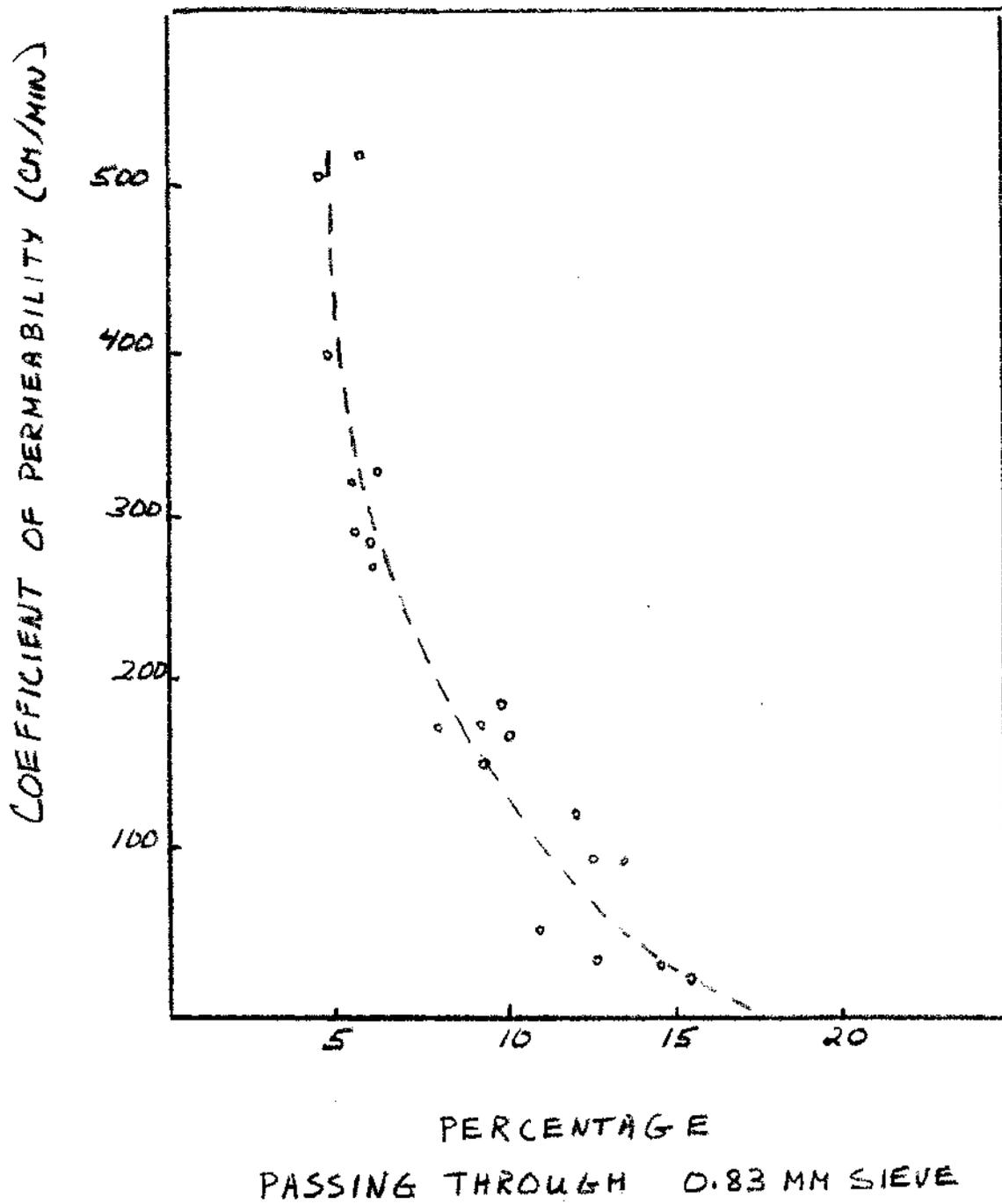
**Figure 1.** Relationship between coefficient of permeability and the fraction of the total volume of the stream bottom materials passing through a 0.83 mm sieve. (Curve fitted by eye). (From McNiel and Ahnell, 1964).
